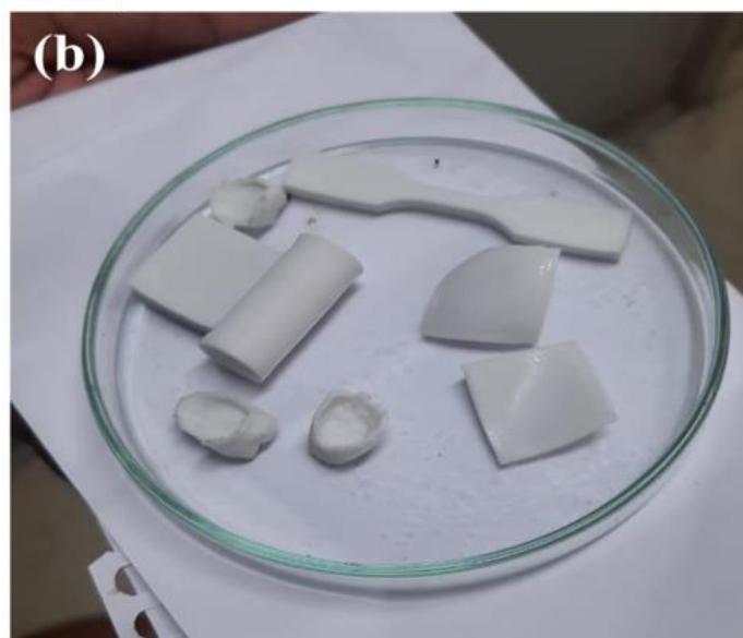
Fig 9(a) Variation of % weight gain after saliva absorption for 30 days, (b) digital image of samples after 30 days of saliva absorption.
