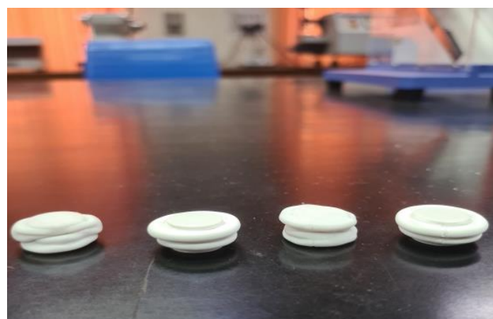
Fig. 7. Post-compression test showing deformation.
